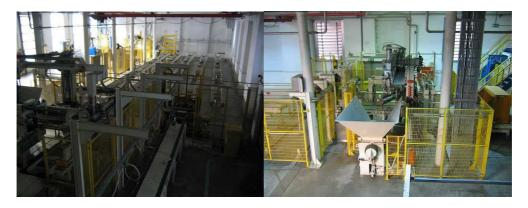
2 x Pulper Grubbens 26m3 with drive motor 250kW
